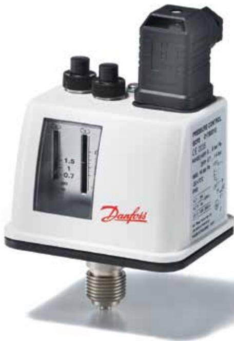
The BCP type is a series of dedicated pressure switches for control, monitoring and safety of steam and hot water boilers. The BCP incorporates a single-pole changeover microswitch where the contact position depends on the pressure in the connection port and the range set value. For installations, in which operation is particularly critical for safety reason, the use of fail-safe control is recommended.
