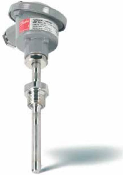
The MBT 5252 is a heavy-duty temperature sensor that can be used for controlling cooling water, lubrication oil, hydraulic oil and refrigeration plants within general industry and marine applications. This temperature sensor is based on a standardized Pt100 or Pt1000 element, which gives a reliable and accurate measurement. NTC/PTC elements available on request.
