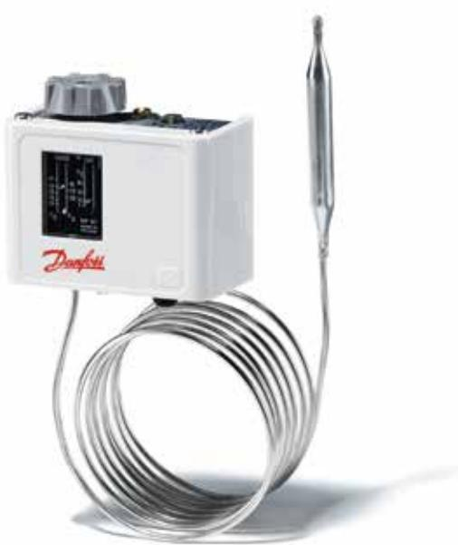
Danfoss KP thermostats are used for control, monitoring and alarm systems in industry. The KP thermostat series are temperature activated electric switches fitted with a single-pole double throw switch (SPDT), which can control single-phase ac motors of up to 2 kW directly.
