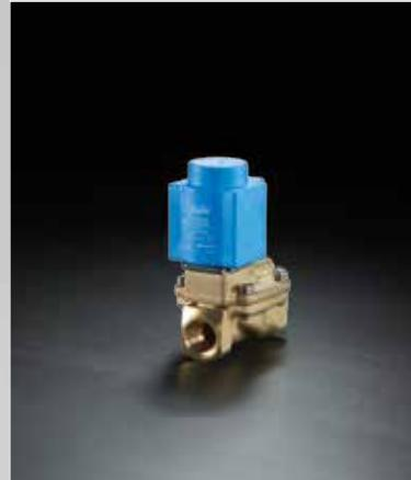
**Externally operated valves** are designed for specialised and demanding applications. These robust valves are the right choice for media with high dirt content, high viscosity, high ambient and media temperatures and large flow volumes. They are also suitable for humid environments, explosion hazard environments and for applications with low or unknown pressure conditions.
